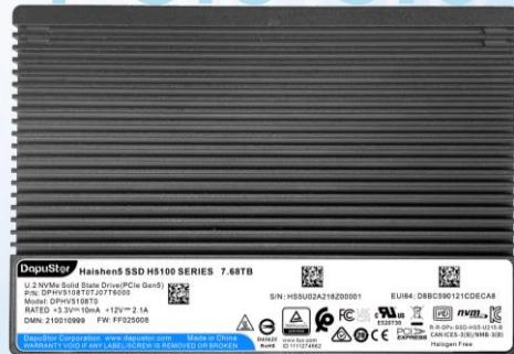
The DapuStor Haishen5 Series adopts the latest Marvell™ PCIe Gen5 enterprise controller named Bravera™ and 3D eTLC NAND Flash with DapuStor in-house firmware. It offers [double throughput compared with the PCIe Gen4 enterprise SSD](#). The DapuStor PCIe Gen5 eSSD is designed for data centers, catering to the increasingly storage demands of different industries, like IT, Internet, Finance, Operators, Smart manufacturing, AI, as well as Oil, Electricity and Energy industries.
